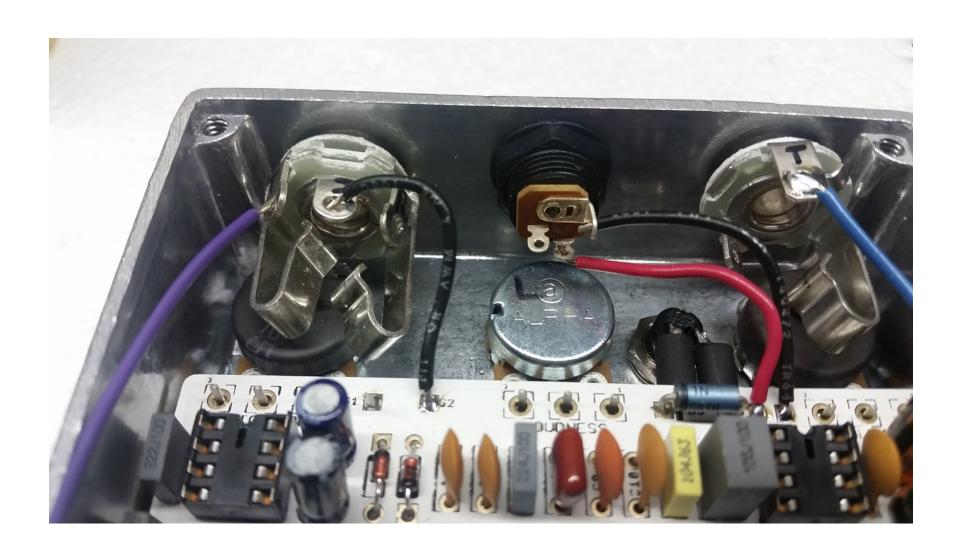
**Step 9:** Install battery, enclosure back and knobs. Knobs will have a small set screw that will need to be tightened with a small flathead screw driver in order to properly operate the potentiometer.
