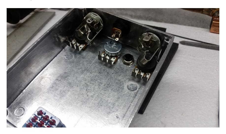
**Step 6:** Time for wiring. Ground wires (G, G1, G2) will be black, power wires (V) will be red and signal wires (I,O) can be any color that is not red or black to avoid confusion. Cut the following lengths of wire:
