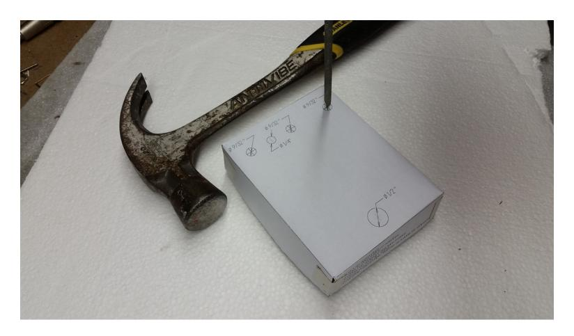
**Step 4:** Drill using the divots as starting points to ensure that the drill doesn't walk off center. Brace the enclosure while drilling to prevent the enclosure from spinning around if the drill catches.
