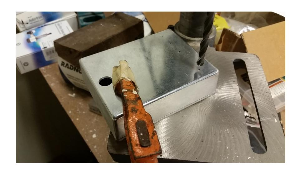
**Step 5:** Use a countersink, if necessary, to de-burr the holes.
